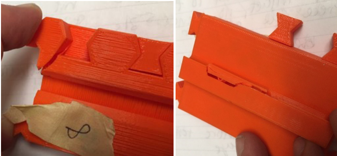
Figure 5: First damage seen in backbone on trial 8. Slight breakage on top attachment but bigger crack on bottom.
