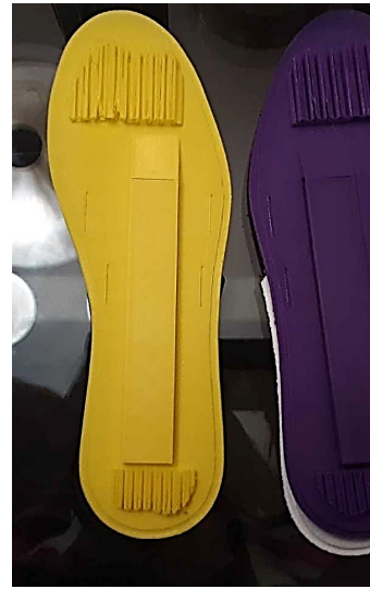
Figure 1. Bottom view of final orthotics
