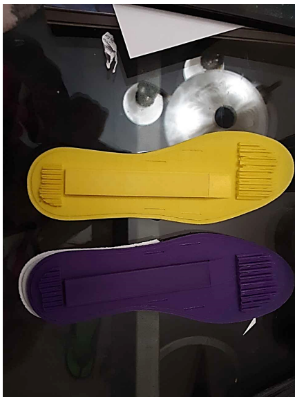
Fig. 1/ Table II. All heights measured in inches then converted into centimeters. The height without the prosthetic was subtracted from the height with the prosthetic to determine how much height was caused by the orthotic. The average height boost is 3.048 cm..
