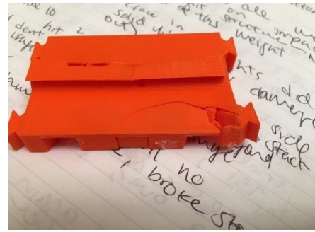
Figure 7: Final Damage to the Backbone. Damaged enough that it couldn't be reused, or stacked back together, but still strong enough and structurally sound enough to support weight and maintain shape.
