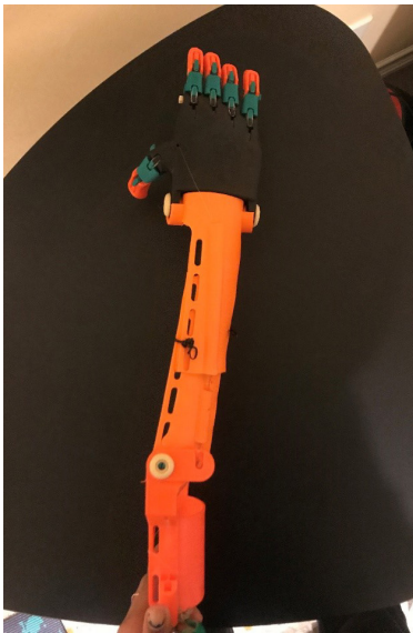
Fig. 1. The measurements of the final design follow two forearm pieces at lengths 5.5 cm and 5 cm. When placed on top of each other the shortest forearm length is 6 cm, the next hole was placed to create a total forearm length of 8 cm and the next hole to create a length of 10 cm. The fishline was strung from the tip of each finger all the way through the arm to the top of the bicep cuff.
