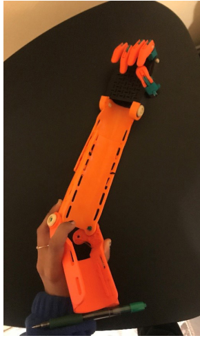
Fig. 3. A body powered mechanism was used. With the string running from top to bottom of the arm, with a bend in the elbow, the string would tighten causing the fingers to close into a fist. With the release of tension in the strings after the elbow was released the fingers would return to normal because of the rubber bands placed in the finger joints.
