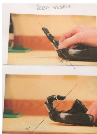
Fig. 1b. Angular displacement of modified model, again using the bottom of the picture as a reference
