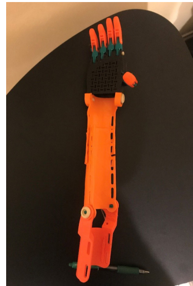
Fig. 2. The measurements of the final design follow the palm size of 2.5 cm and a bicep cuff of 4.5 cm. All pieces were attached with washers and pins at each connection point. The fingers were assembled and at each joint, orthodontic rubber bands were wrapped around to create a tension mechanism.
