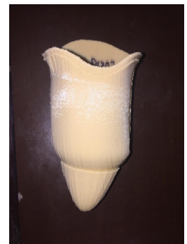
Figure 4: The top view of the first prototyped 3D-printed socket prosthetic.
