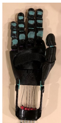
Fig. 2b. Final model assembled without bottom Velcro strap in order to show cable system running through the hand.
