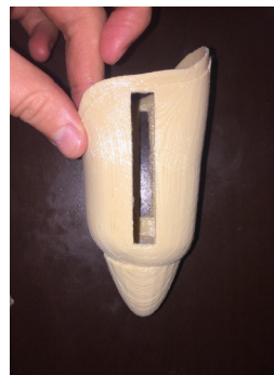
Figure 3: The side view of the first prototyped 3D-printed socket prosthetic, showing off the longitudinal slits on each side.
