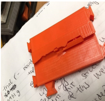
Figure 6: Small dent next to top attachment piece, still structurally sound. Trial 10.
